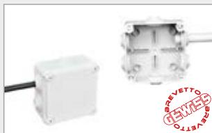
The boxes fitted with cable glands make it possible to quickly insert rigid and flexible cables between  $\varnothing$  4 and 14 mm and rigid conduits. The innovative geometry guarantees high mechanical performance and ensures the maintenance of the degree of protection of the box, also with the cables or conduits inserted.
